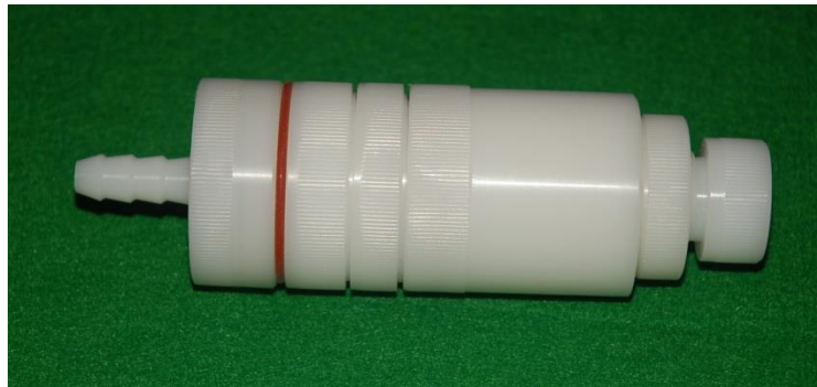
Filter pack ready to be sampled by means of an external pump
