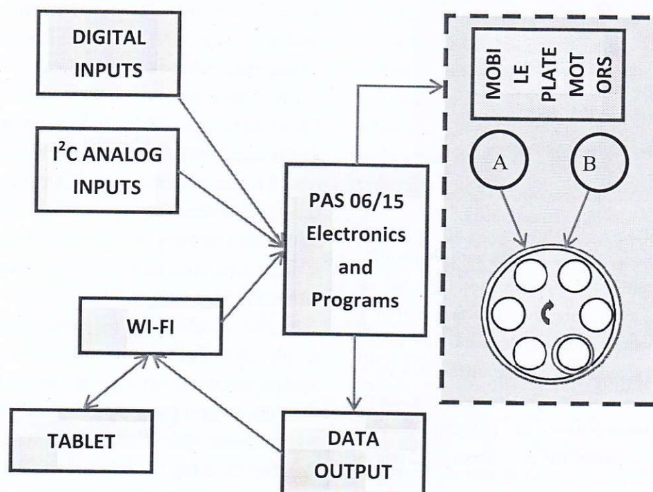
Fig. 3 Electronics and interfaces of the sampler.
