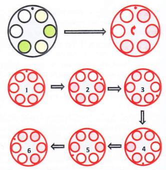
Fig. 2 Sampling sequence for two pairs of passive samplers in two different time intervals.
