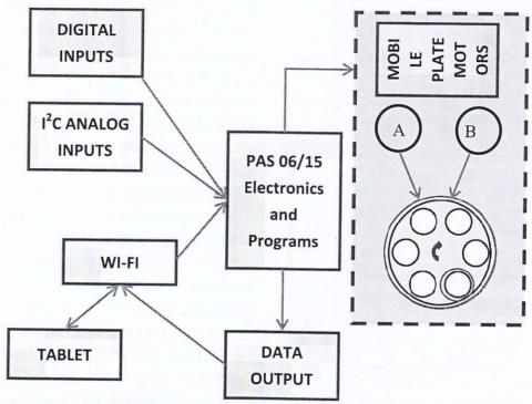
Fig. 3 Electronics and interfaces of the sampler.
